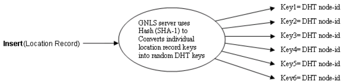
Figure 8: Illustration of GNLS server generation of location records
